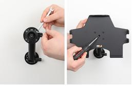
2. Place the attaching plate onto the desired position. Screw the attaching plate into place with the enclosed screws. Place the holder over the attaching plate so the screw fits in the hole in the tilt swivel. Tighten the screw until the holder is firmly in place, but still can be adjusted.
