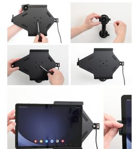
1. Loosen the screw in the center of the holder so you can remove the tilt swivel attaching plate on the back. Place the attaching plate onto the desired position. Screw the attaching plate into place with the enclosed screws. Place the holder over the attaching plate so the screw fits in the hole in the tilt swivel. Screw the holder onto the attaching plate. Tighten the screw so the holder is firmly in place, but still can be adjusted.
