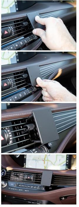
1. Use the enclosed alcohol pad to clean the area where the mount will be installed. Peel off the adhesive tape cover. Place the mount by the right side of the air vent so the short side of the upper and lower parts are toward the driver's side. Hook the upper edge under the frame surrounding the air vent.
