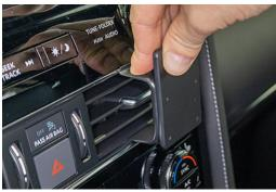
3. Press downward and forward on top of the mount. Hook/Clip the upper edge into the gapbetween the air vent housing and the dashboard panel.
