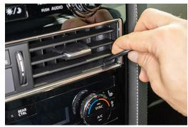
1. Press the included gap opener into the gap between the air vent housing and the surrounding dashboard panel, to widen the gap.
