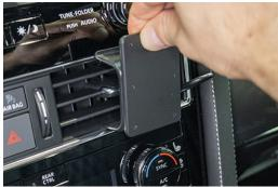
2. Press the lower edge of the mount into the gap next to the gap opener. Pull out the gap opener.
