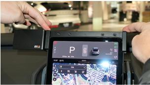
2. Slowly and firmly, press down on both sides of the mount to slide/hook it onto the screen.
