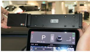
1. Choose if you prefer to have the device installed on the driver's or passanger's side of the screen, and place the face plate onto the corresponding side of the mount. Make sure the face plate is on the correct side and attach it to the mount base with the included screws (Phillips screwdriver). Place the mount above the screen.
