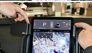
3. Press downward until the mount is securely in place.
