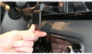
3. Press upward on the lower part of the mount so the edge goes all the way into the gap. Pull out the gap opener.
