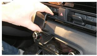
1. Press the thin end of the included gap opener into the gap between the control panel and the dashboard, to widen the gap. Use the enclosed alcohol pad to clean the area where the mount will be installed. Peel off the adhesive tape covers. Hook the upper edge of the mount over the frame surrounding the air vent.
