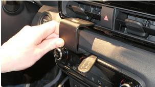
2. Pull the lower part of the mount downward and hook the edge into the gap next to the gap opener.
